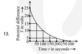
The figure shows an experimental plot for discharging of a capacitor in an R-C circuit. The time constant  $\tau$  of this circuit lies between :
